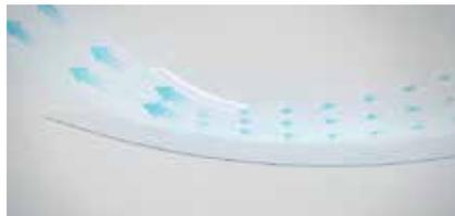
The optimal pressure expansion duct that is narrow inside and wide outside between dual layers where Venturi Effect occurs when air flows through the duct. Thus, the airflow is instantly released at high speed.
